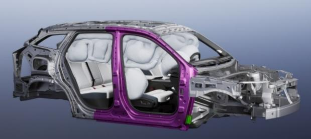
The steel frame provides unparalleled protection for occupants, thanks to its 32000Nm/°torsional durability. In the event of a collision, the steel frame absorbs and distributes forces efficiently, minimizing the impact on passengers.
