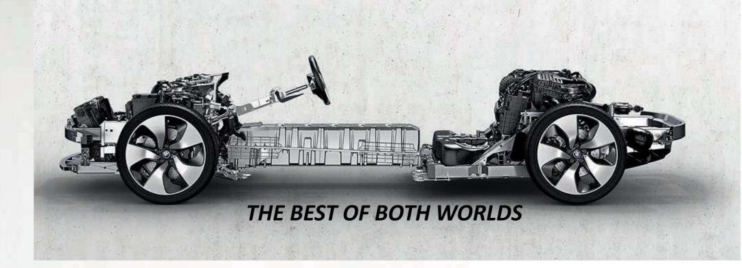
WITH THE ELECTRIC MOTOR AT THE FRONT AXLE
